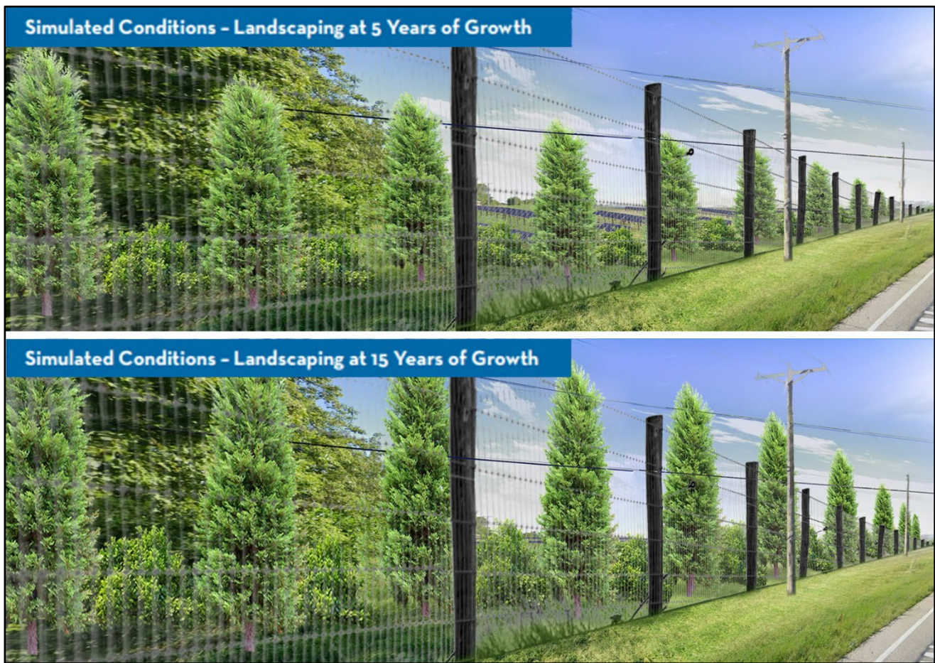
Photo 8. Rendered Image of Vegetation Buffer, Fixed Farm Knot Fence (8 ft tall) and Solar Panels (50 feet setback back property line. Simulated at 5-year growth and 15-year growth.
